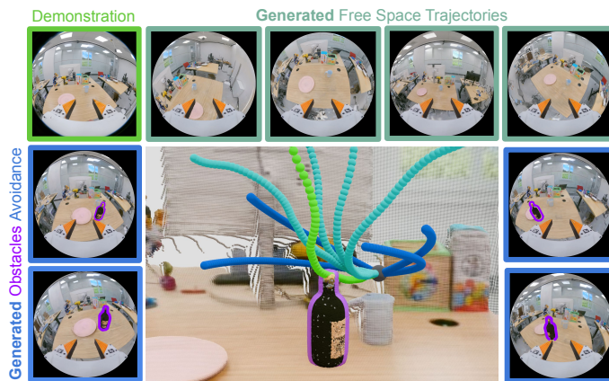
Fig. 1: 1001 DEMOS. From a single human demonstration (e.g., picking up the blue mug), our approach generates valid training trajectories with large spatial variance and augmented obstacles , while respecting action-view consistency, 3D collision and contact dynamics constraints.
